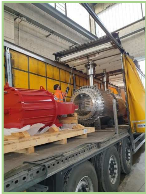
Big Low-Noise Control ball valve for Natural Gas ready to be shipped
